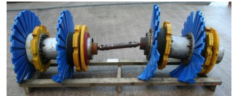
24" / 34" dual diameter pig
