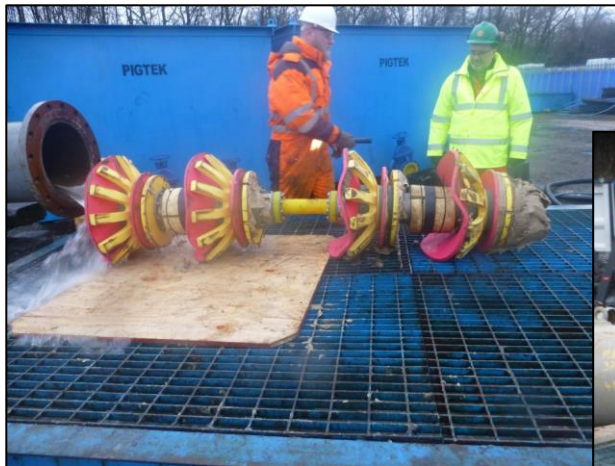
16/24E being recovered from 16" pipe follow wax and compression trial
