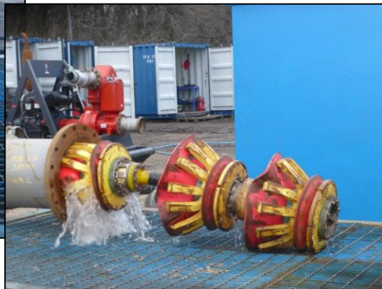
16/24E being recovered from 16" pipe follow wax and compression trial
