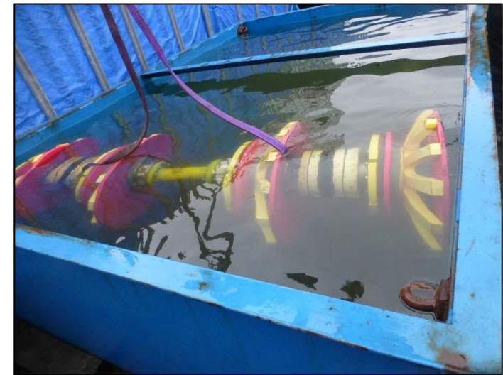
16/24E pig neutral buoyancy check in test tank
